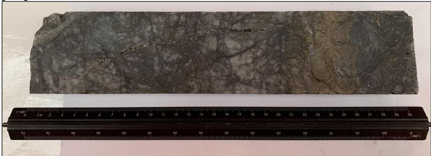
Figure 2: Split section of drill core from hole FR-DD-22-UG-187 grading 38 g/t Au and 54 g/t Ag over an estimated true width of 0.18 metres.
